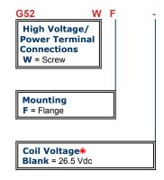
\*Order the relay with the coil voltage in the part number as shown above. The coil voltage will appear on the coil plate near the coil terminals rather than in the P/N on the relay.
