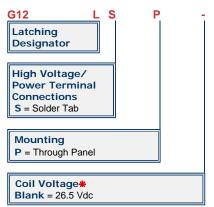
Order the relay with the part number as shown. The latching "L" designator and the coil voltage will not appear in the P/N on the relay but will be indicated on the label that is on the base of the relay. Observe coil polarity.
