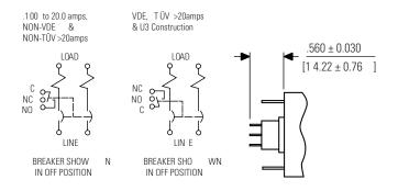
Note B: Switch is located in the left hand pole (viewed from terminal end).
