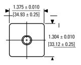
Mounting Detail (Single Pole and Two Pole)
