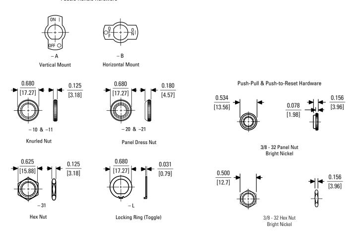
Note: Tolerance ± .010 [.25] unless noted. Dimensions in brackets [] are millimeters.
